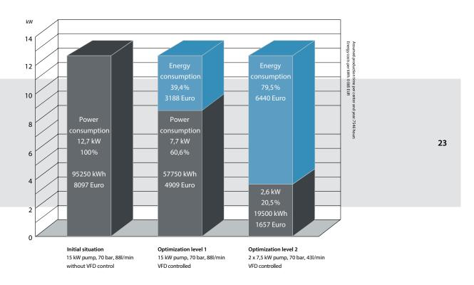
STAMA has implemented innovative ideas for more efficient energy use. One is the use of frequency-controlled cooling lubricant pumps. These cut energy costs by a good 80%.
