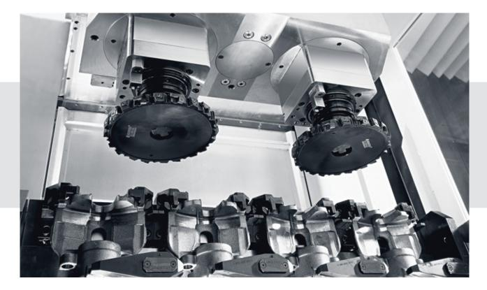
The target application of multi-spindle machining defines the particular basic properties of the TWIN and TWIN<sup>2</sup> machining centers from STAMA: high thermal-mechanical stability and rigidity.
